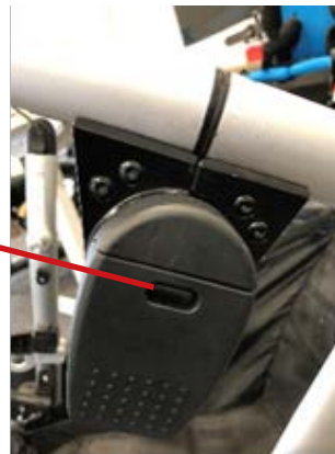
T Bolt is not damaged
